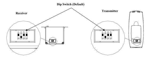
Do not use two (2) or more remote control systems in the same area with the same dip switch settings, as they will communicate with each other. This may cause the appliances to malfunction.
